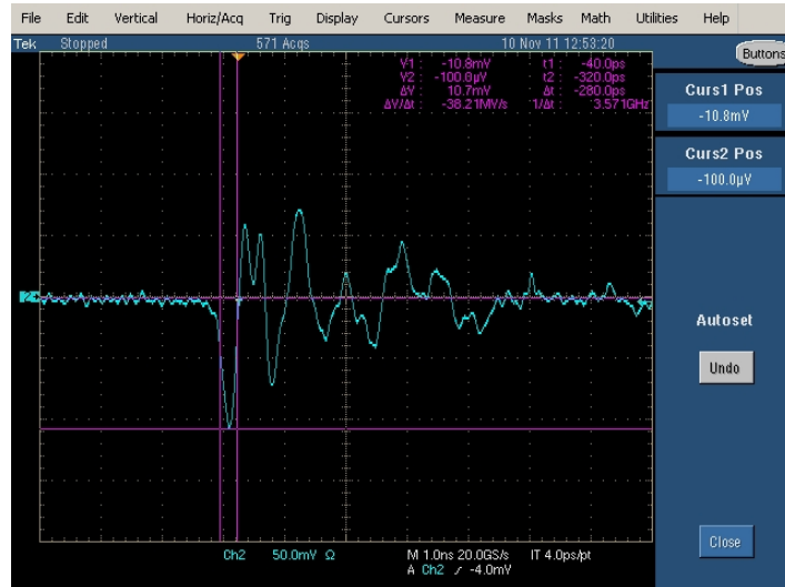
Fig. 3.4.2b The voltage signal is observed on oscilloscope using ring-antenna detector at which the copper diameter is 0.53 mm.
