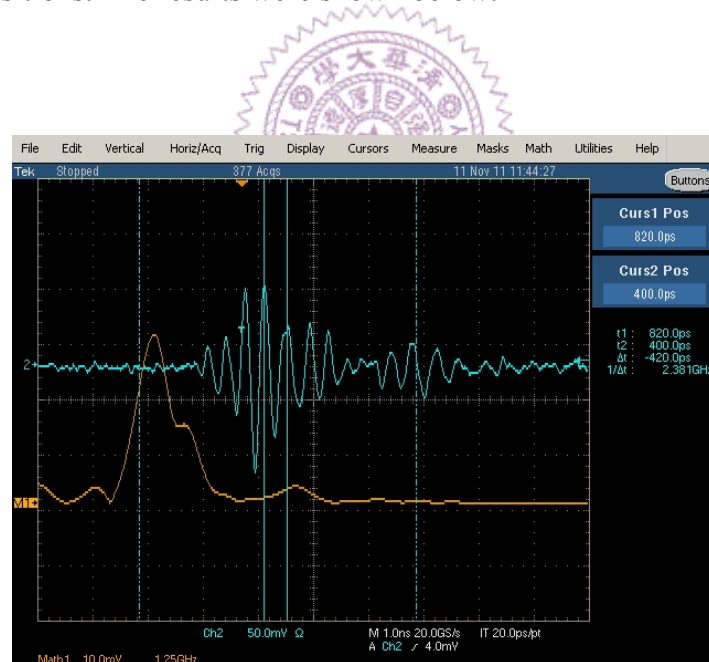
Fig. 3.4.7 The E-field polarized along vertical horizontal and the ring-antenna was put after the directional coupler. The blue curve was the signal detected by the ring-antenna and the orange curve was the FFT result.
